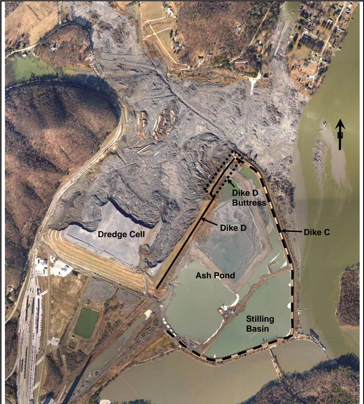
Figure 1. Kingston Fossil Plant Dredge Cell Failure (photo from TVA)
